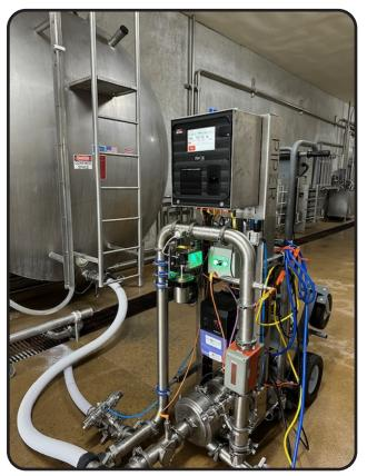
hours, varying according to the tank's size. In addition, there should be an ample supply of water to completely fill the milk tank. To ensure precise calibration, water is systematically metered into the tank in small increments, allowing it to settle completely before measurement. The measurements are then recorded into a new calibration chart. This procedure guarantees accurate and reliable calibration results.
